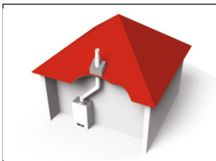
Figure 1.3.2 Maximum equivalent length: 6 m
